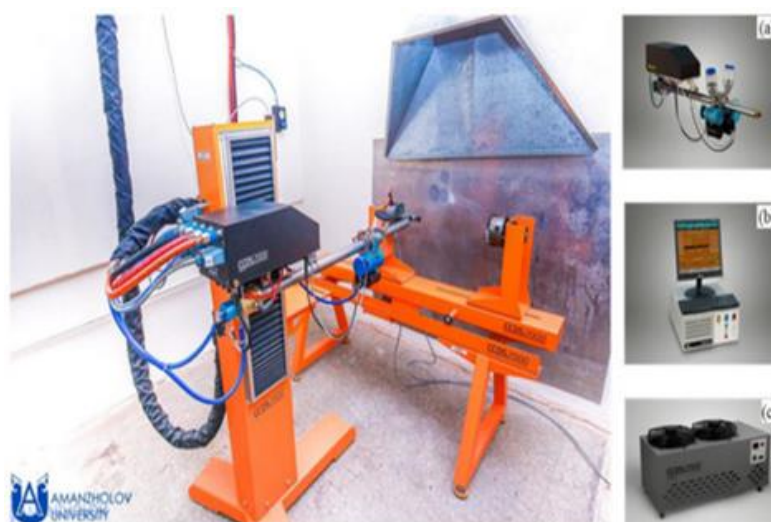
Fig. 1. CCDS2000 computerized detonation complex: (a) detonation barrel, (b) control unit, and (c) cooling system.
